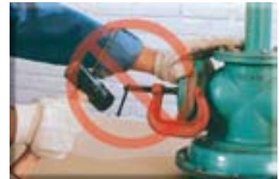
**Never strike the lever to try to add more pressure to the clamped object.**
