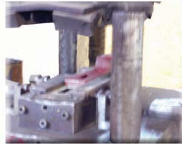
2. Hot die-casting (Punched and Bent into the Claw)
