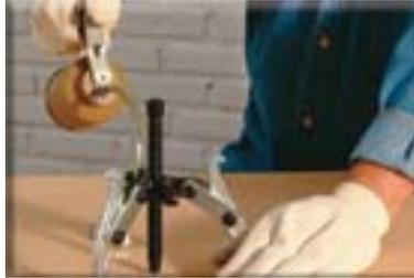
**Always make sure that the center screw is clean and well lubricated.**
