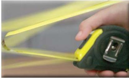
Use the touch braking system (manual pressure) to prevent accidents when retracting the tape back into the tape measure.
