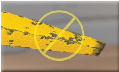
Dispose of any pry bar that is damaged, cracked, or has an excessively worn claw.
