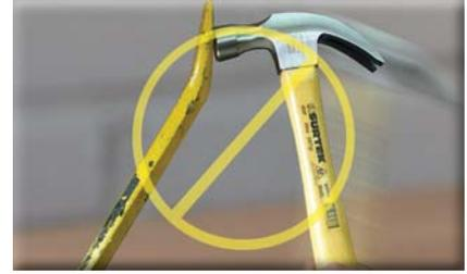
Never use a hammer to hit a claw bar; it could splinter.
