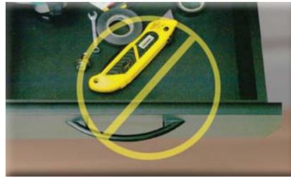
Do not store a retractable knife without retracting the blade.
