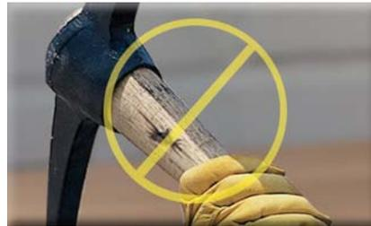
Never use a pickaxe that is damaged or has cracks in the handle.
