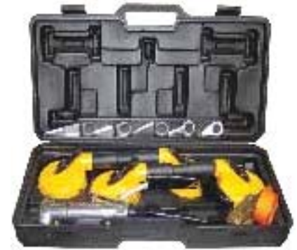
AIR WINDSHIELD REMOVAL KIT Pneumatic windshield knife with suction cups. Kit includes: windshield knife: 20,000 oscillations per minute, rear exhaust, teasing throttle and regulator provide easy speed control, flexible 12 position blade mount, includes 5 blades, suction cups: (2) 4 5/8" diameter double suction cups. Ratcheting tie down molded storage case. Stock No. 684
