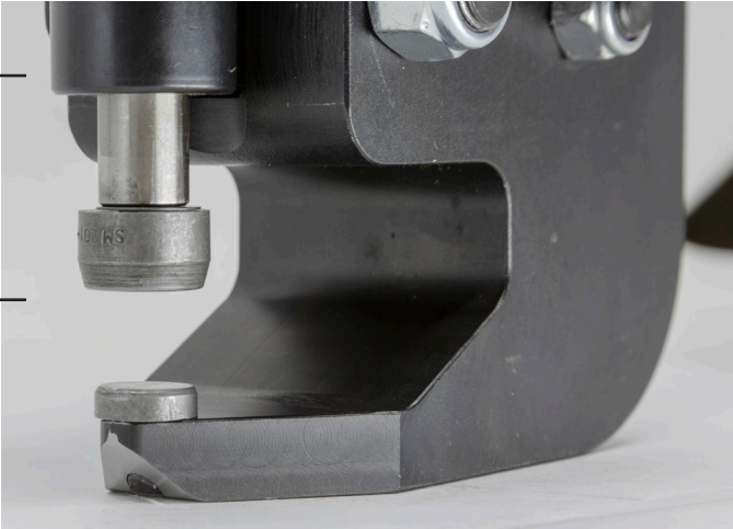
Rivet set holder P073237 & rivet set are in forward position due to return piston adjuster bolt.
