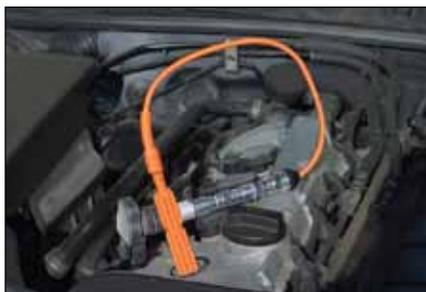
Test coil directly to ground
