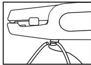
1. To cut wire, place wire to desired length between cutter blades and squeeze handles.
