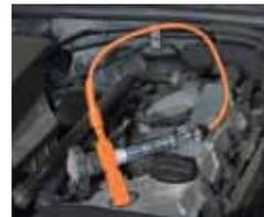
Shown testing vehicle with recessed spark plugs
