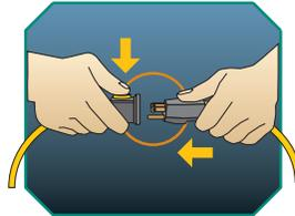
**TO LOCK** a plug to your new Push-Lock® extension cord, depress the oval button on the receptacle and insert tool blades and ground pin of tool plug. You will hear the locking mechanism engage.
