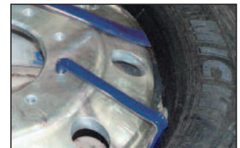
• Curved end For mounting and demounting top bead
