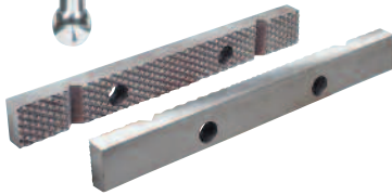
"V" notched, replaceable/reversible jaws made of carbon steel and heat-treated for extra strength, diamond cut on one side - smooth on the other
