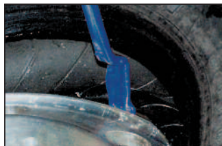
• Bent end For mounting and demounting bottom bead
