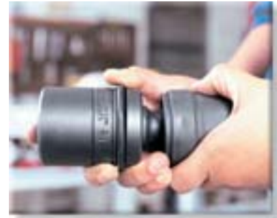
Step 3: Finally, place the retaining ring in the channel on the impact socket.
