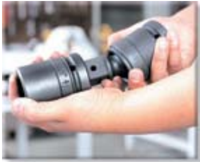
Step 1: Insert the accessory to be used into the impact socket
