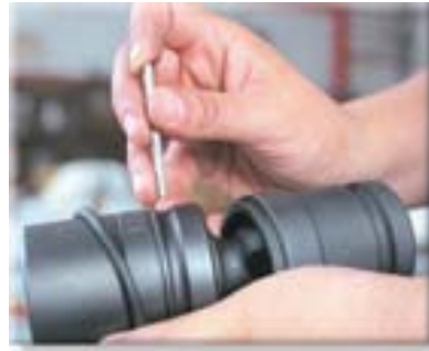
CODE 10000RX and 10000PX O-rings and pins for 1" impact sockets and accessories Step 2: Insert the retaining pin into the socket that goes through the accessory's male drive.
