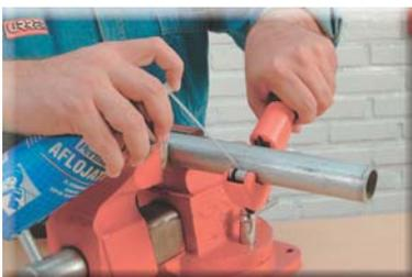
The pipe and pipe cutter should be lubricated to reduce friction.
