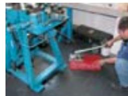
3. Pump the liquid into the circuit until it reaches the pressure comprobation.
