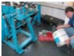
2. Fill the circuit with liquid and extract the air, close hermetically all the openings.
