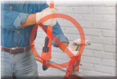
Never use a pipe wrench to bend, hoist, or lift a pipe.
