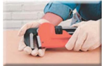
Clean and inspect pipe wrenches periodically. If damaged or broken teeth are found, the jaws should be replaced.
