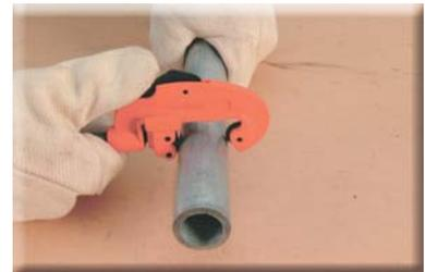
When using a pipe cutter, always mount it perpendicular to the pipe.
