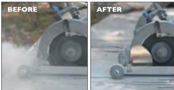
VACUUM REQUIREMENTS: SawVac™ will work with any vacuum, but for optimum efficiency use a vacuum rated at or above 11.5 amps (1.75 continuous hp) or 110 cfm.
