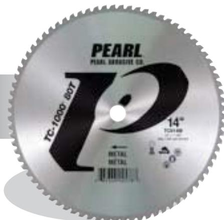
Pearl's Titanium Carbide Tip Metal blade (TC-1000™) is designed to cut a variety of mild ferrous metals with fewer burs, less dust and reduced material burning than abrasive products. It provides much longer life than traditional abrasive wheels. The Pearl TC-1000™ is engineered with a triple chip design for added durability.
