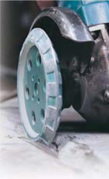
FOR CLEANING, ROUTING AND REPAIRING OF CRACKS IN CONCRETE AND MOST OTHER BUILDING MATERIALS.
