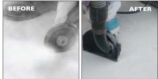
VACUUM REQUIREMENTS: QuikAttach™ will work with any vacuum, but for optimum efficiency use a vacuum rated at or above 11.5 amps (1.75 continuous hp) or 110 cfm.
