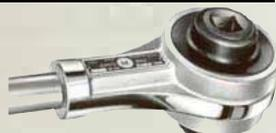
The X-4 Torque Multiplier is a Geared Head Wrench incomparable to any other tool. The multiplication is achieved through a planetary gear train at a 4:1 ratio (or other) depending on the model. It generates torque's from a few hundred pound-feet to thousands of pound-feet with precision and ease.
